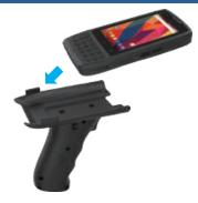
1. Install the Rugged Handheld on the Scanning Trigger.
