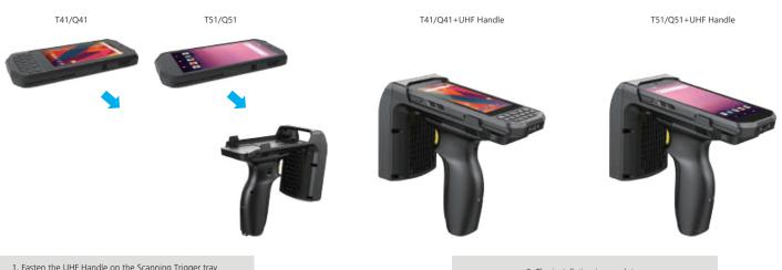
1. Fasten the UHF Handle on the Scanning Trigger tray in the direction shown in the figure.
