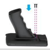
2. Align the two holes on the top of the Scanning Trigger with the two holes beside the battery lock on the back of the Rugged Handheld.
