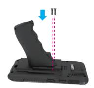
2. Align the two holes on the top of the Scanning Trigger with the two holes beside the battery lock on the back of the Rugged Handheld.
