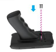
2. Align the two holes on the top of the Scanning Trigger with the two holes beside the battery lock on the back of the Rugged Handheld.
