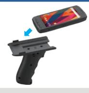
1. Install the Rugged Handheld on the Scanning Trigger.
