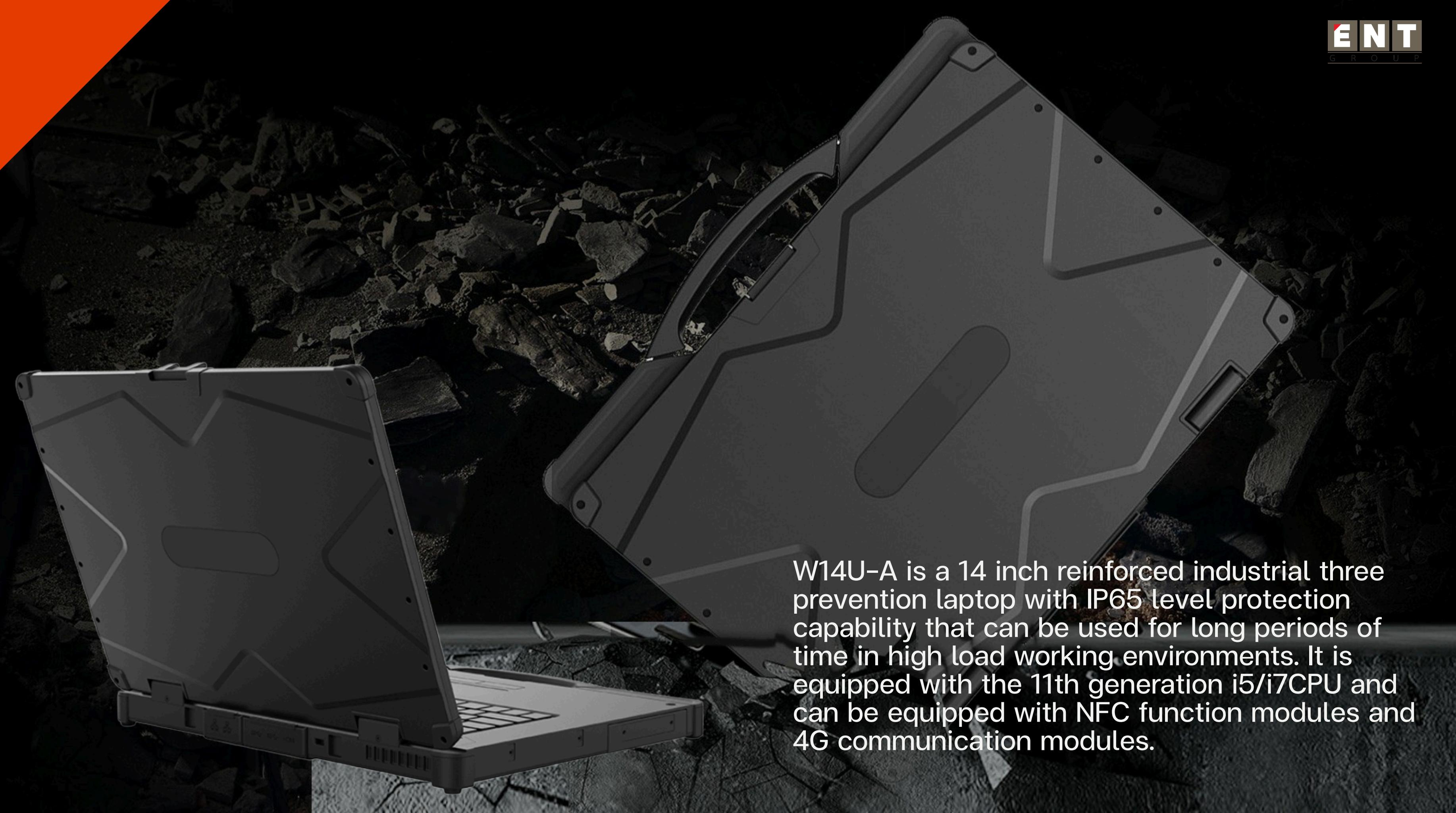
W14U-A is a 14 inch reinforced industrial three prevention laptop with IP65 level protection capability that can be used for long periods of time in high load working environments. It is equipped with the 11th generation i5/i7CPU and can be equipped with NFC function modules and 4G communication modules.
